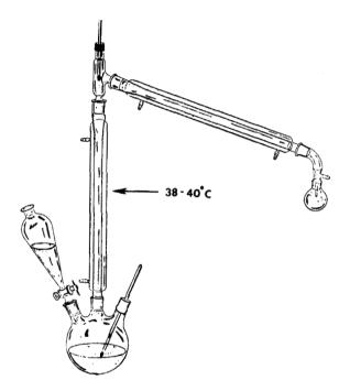
remained between 130-160° throughout the reaction and the  $\underline{t}$ -butylacetylene was collected at a rate of about 1 drop every two seconds. The crude  $\underline{t}$ -butylacetylene was fraction-ally distilled, bp. 37-39°, to yield 62.1 g (89%). Its nmr spectrum was consistent with that expected.<sup>4</sup>
